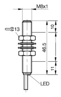
Inductive Sensors BES 516-324-EO-C-02 M8x1 x 46.5 normally-open Sn=1,5mm shielded
